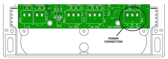
The power connection (CN8) is a three wire terminal block located on the far right. Two terminal screws marked AC are for connecting to a low-voltage source, isolated from earth ground. See section 2.0 Specifications for power source requirements. Due to the low power requirements of this console, a 16 or 18 AWG wire would be sufficient for these two power connections.
