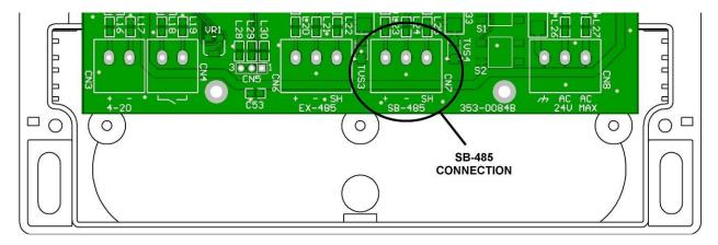
The SB-485 connection (CN7) is a three wire terminal block located near the center of the printed circuit board and is for connection to the SmartBob RS-485 network. Two terminal screws marked + and – should be connected to the positive and negative wires of the SmartBob network cable. The third terminal screw marked SH should be connected to the shield of the SmartBob network cable. Do NOT connect the shield to earth.
