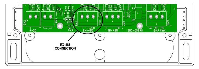
The EX-485 connection (CN6) is a three wire terminal block located near the center of the printed circuit board and is for connection to the Expansion RS-485 network. Two terminal screws marked + and – should be connected to the positive and negative wires of the RS-485 network cable. The third terminal screw marked SH should be connected to the shield of the RS-485 network cable. Do NOT connect the shield to earth.
